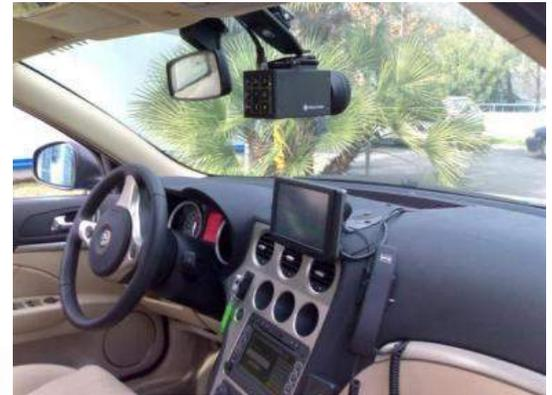
Vehicles used for transport of prisoners or witnesses are equipped with an in-vehicle PC, for Video Transmission, recording and check of number plates following the Patrol car.
